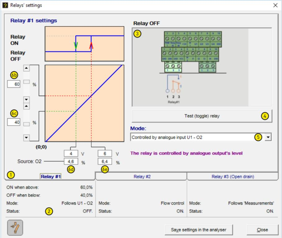
The screenshot shows the 'Relays' settings window. The 'Relay #1 settings' tab is selected. It features a graph with 'Relay ON' (blue line) and 'Relay OFF' (red line) levels. The ON level is set to 60% (6d) and the OFF level to 40% (6e). The source is O2. The mode is 'Controlled by analogue input U1 - O2'. A 'Test (toggle) relay' button is present. The status of Relay #1 is OFF. The window also includes a terminal block diagram and a 'Save settings in the analyser' button.
