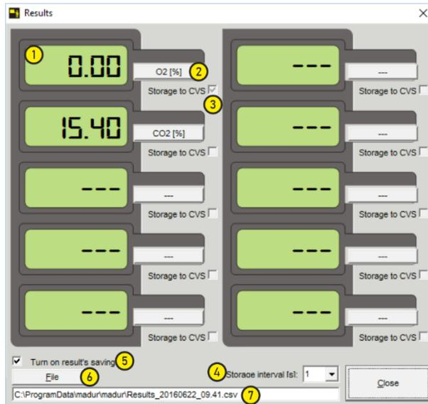
This window allows to view results (independently from device display) and to store them directly to CSV file on hard disk (under condition that this window is active)
